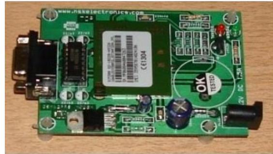
Figure 2: GSM Module.
