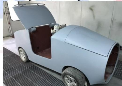
Figure 7 : Primer coat applied after grinding
