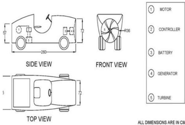
Figure 10: Final draft of the wind powered car
