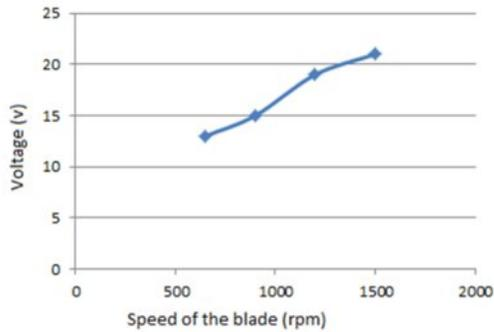
Figure 12: Blade speed vs. Voltage
