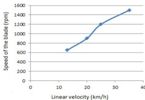
Figure 14: Linear velocity vs. Blade speed
