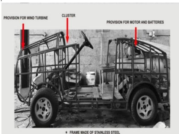
Figure 4: Frame work of the vehicle
