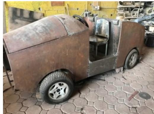
Figure 5: Body work of the vehicle
