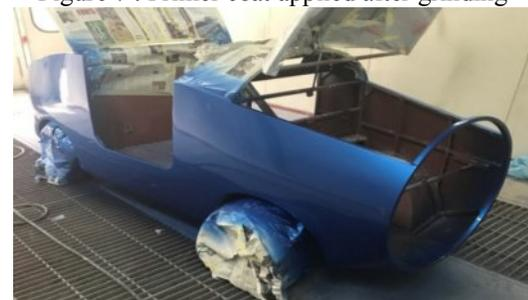
Figure 8: Painting work of the vehicle
