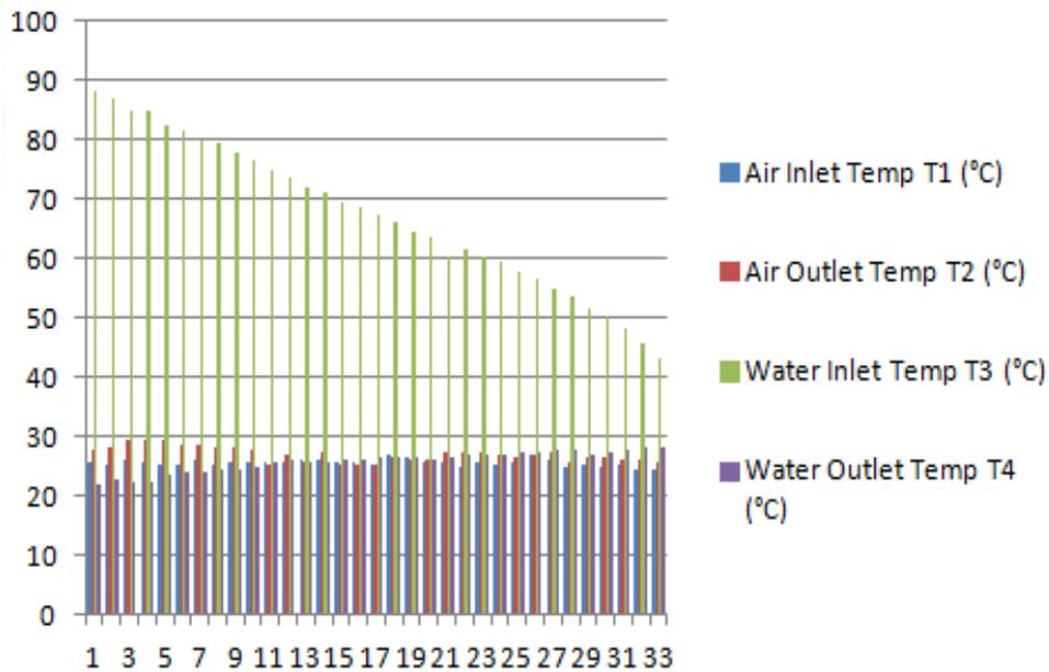
Figure 18: Temperatures at different points when the working substance is water
