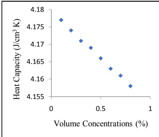
Figure 16: Results of Heat capacity vs. volume concentrations
