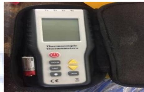
Figure 4: 4-Channel K-Type Digital indicator and thermocouple
