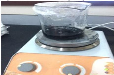
Figure 13: MWCNT being mixed in water using magnetic stirrer method.
