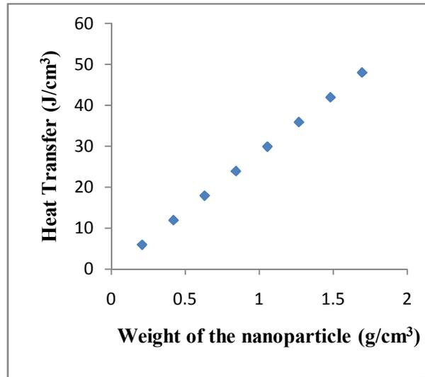
Figure 17: Heat Transfer with respect to weight of nano particle
