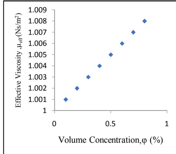
Figure 14: Results of viscosity change with respect to volume concentration of nanoparticle. A figure infers that as volume concentration increases the effective viscosity also increases [3,10].
