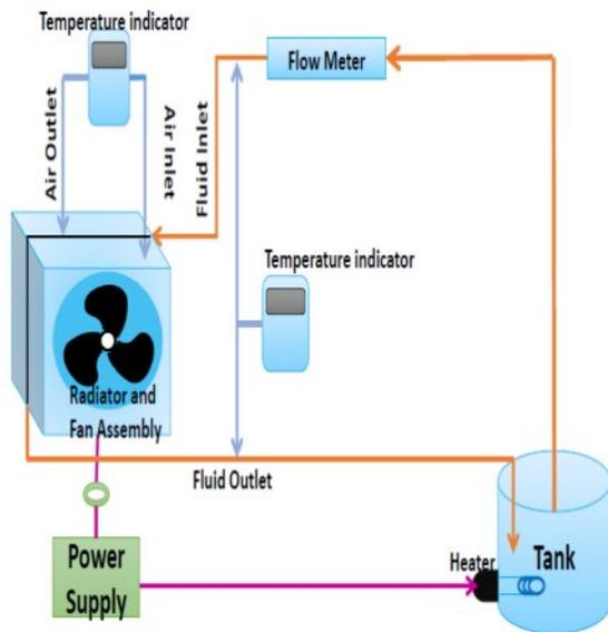
Figure 2: Schematic diagram of the test rig
