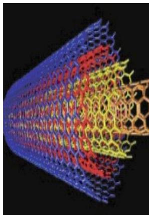
Figure 10: MWCNT Structure
