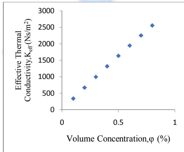
Figure 15: Results of thermal conductivity with respect to volume concentrations
