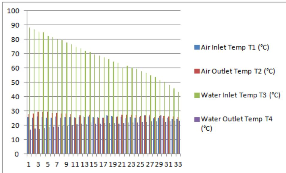
Figure 19: Temperatures at different points when the working substance is water mixed with nano particles
