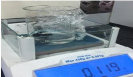
Figure 12: MWCNT being weighed
