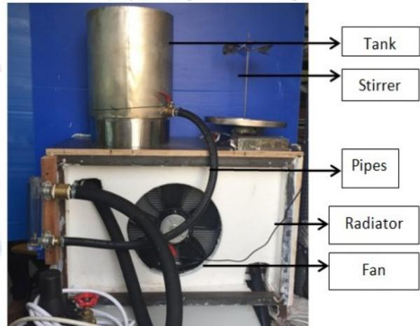
Figure 11: Assembled Test Rig setup (using Gravity Method)
